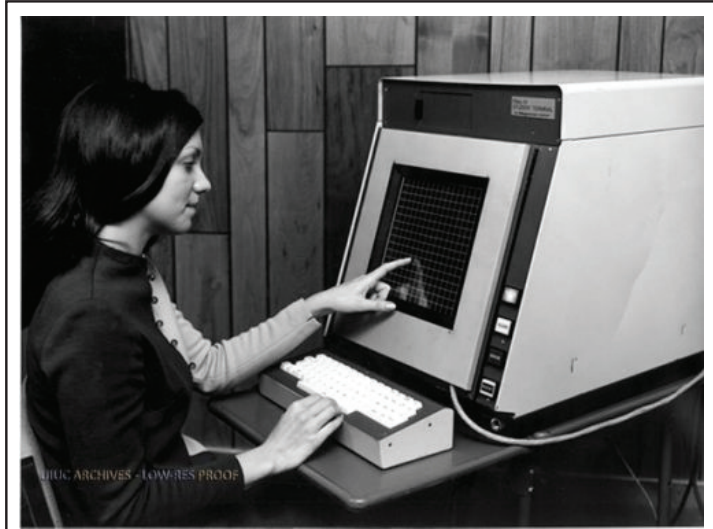
Figure 2: The image above displays one of our world’s earliest touch screens. When touching a screen, the body acts as an electrical conductor and completes a circuit. This disrupts the flow of electricity at the point that has been touched and the computer is able to register the location of touch on the screen.
