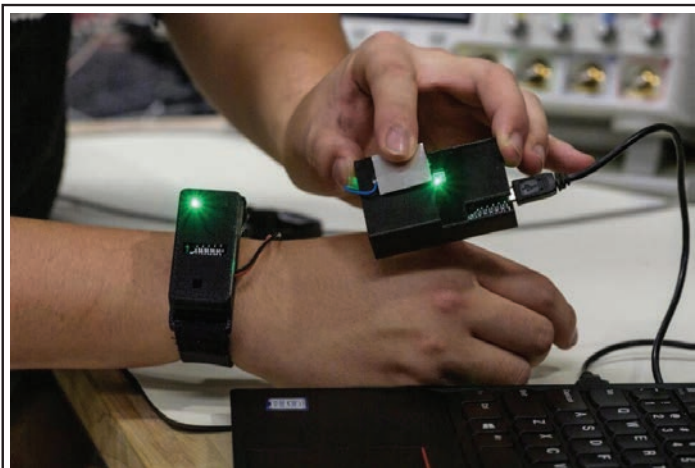
Figure 3: The picture above shows a moment during Purdue University’s experimentation. Information from a chip in the man’s watch is being transferred to the computer as the man touches the receiving sensor. The body behaves as an invisible wire that allows the information to flow from the watch to the computer.
